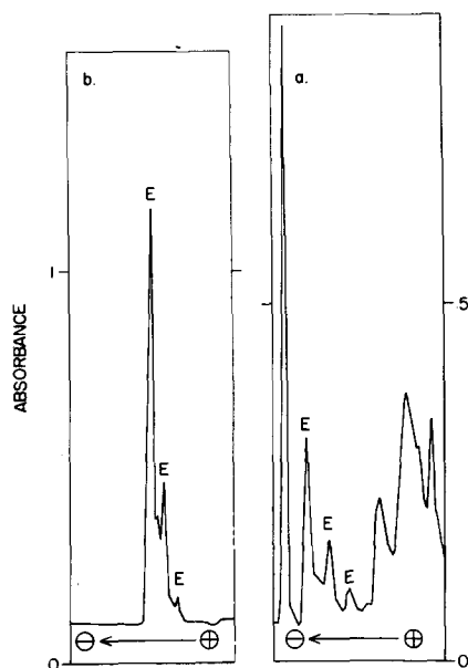
Fig. 5. Scans of acrylamide disc gel electrophoretograms. a, low salt (0.10 M NaCl) crude granular extract, 130 \mu g protein; b, elastase, 45 \mu g protein. Both stained with Buffalo Black stain. See text for details.
